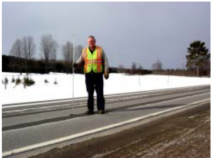
Foreman Randy Thompson inspects the "Frost Tube", February 2011
